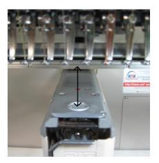
You can use the Passivity Knob that you see in the picture to the right to correct the error by rotating the knob clockwise or counterclockwise until you can align the needle with the hole on the needle plate.
